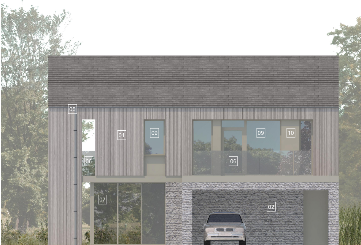
ELEVATION 03 EAST ELEVATION
