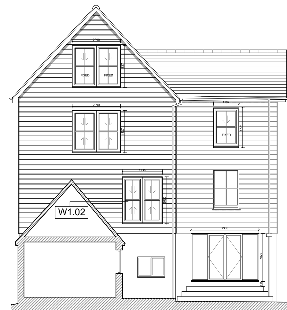
PROPOSED SOUTH ELEVATION SHOWING HIDDEN WINDOWS [south] 1:100
