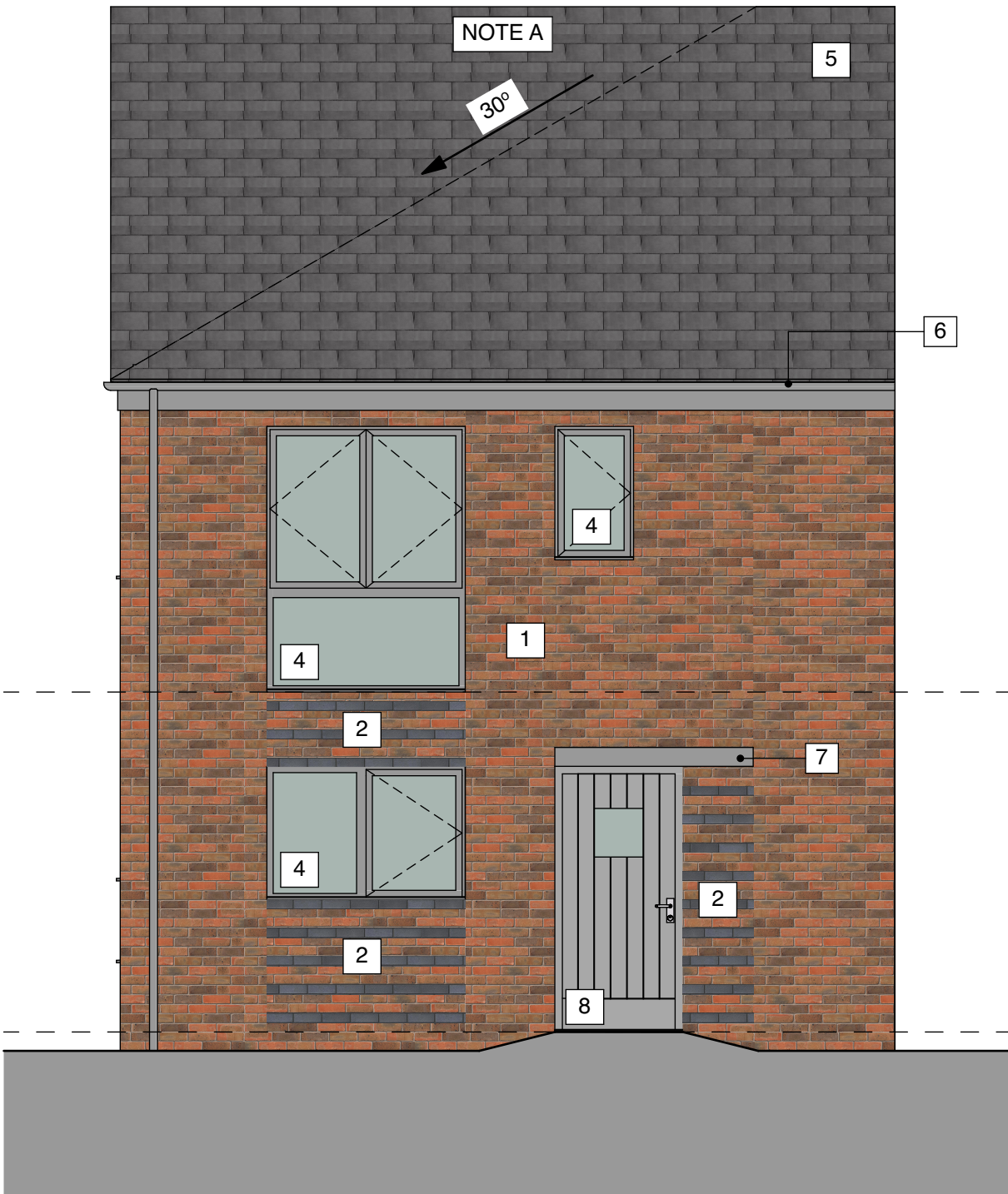
Front Elevation - Facade Treatment B
