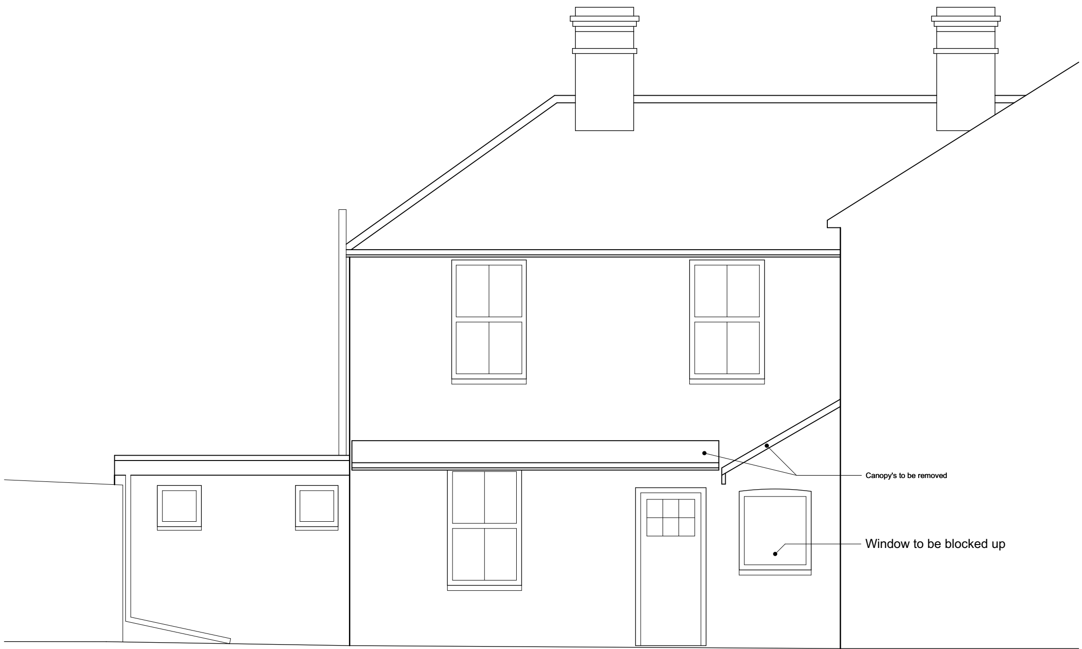
Existing North Elevation 1:50
