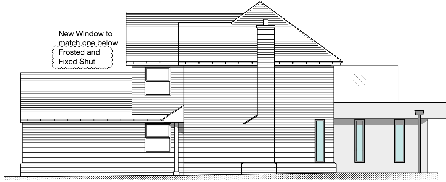
SIDE ELEVATION [north] 1:100
