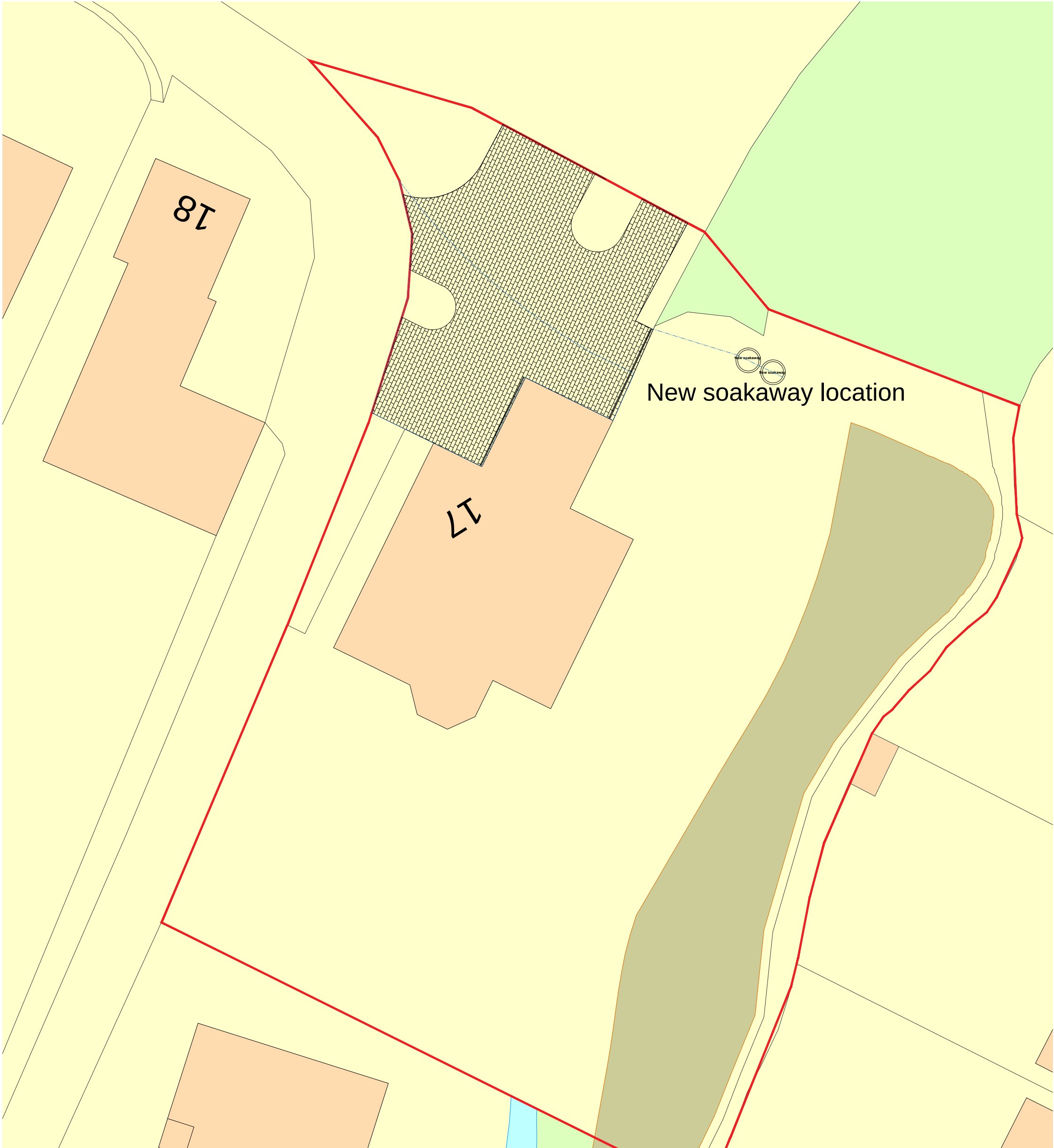
Installed driveway area - 180 Sq M with additional remedial soakaway. Ordnance Survey, (c) Crown Copyright 2019. All rights reserved. Licence number 100022432
