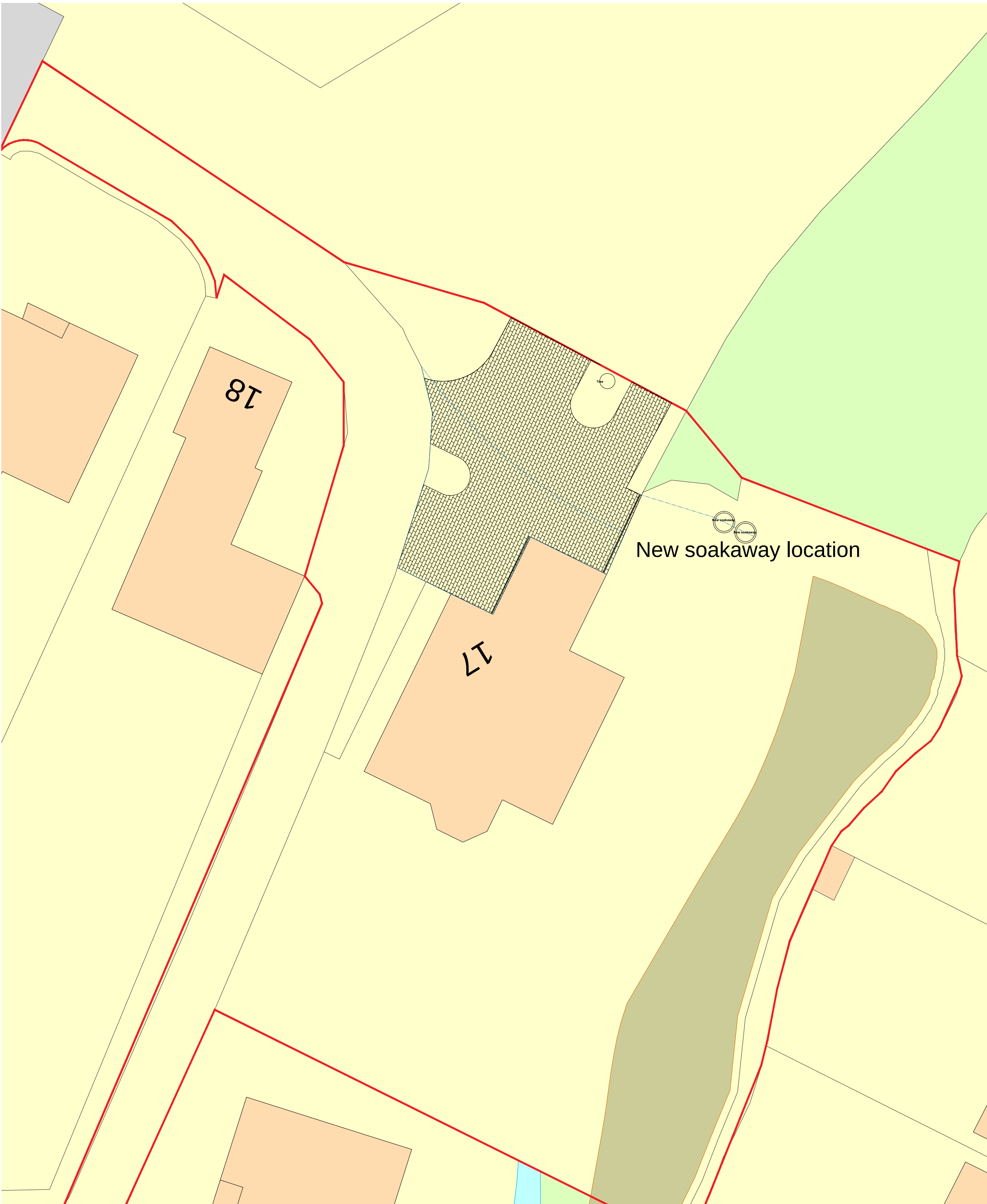
Installed driveway area - 180 Sq M with additional remedial soakaway. Ordnance Survey, (c) Crown Copyright 2019. All rights reserved. Licence number 100022432
