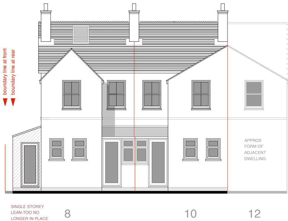
Existing SOUTH (Rear) Elevation at 1:100 scale
