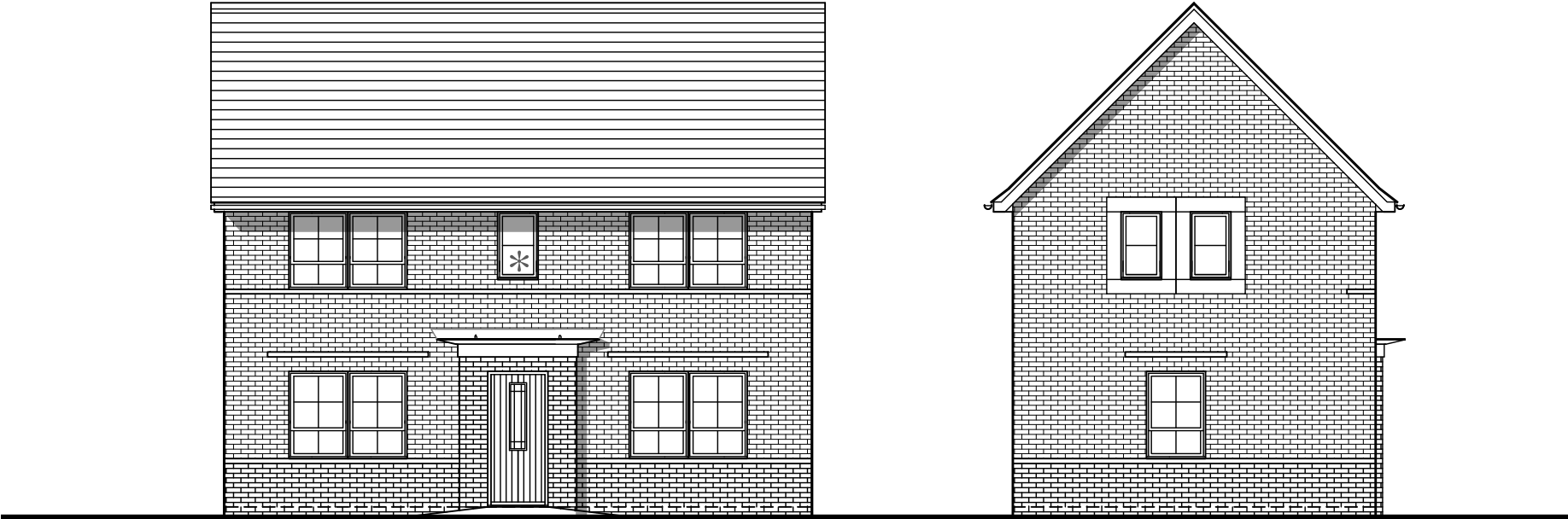
FRONT ELEVATION * Obscure Glazed Windows
