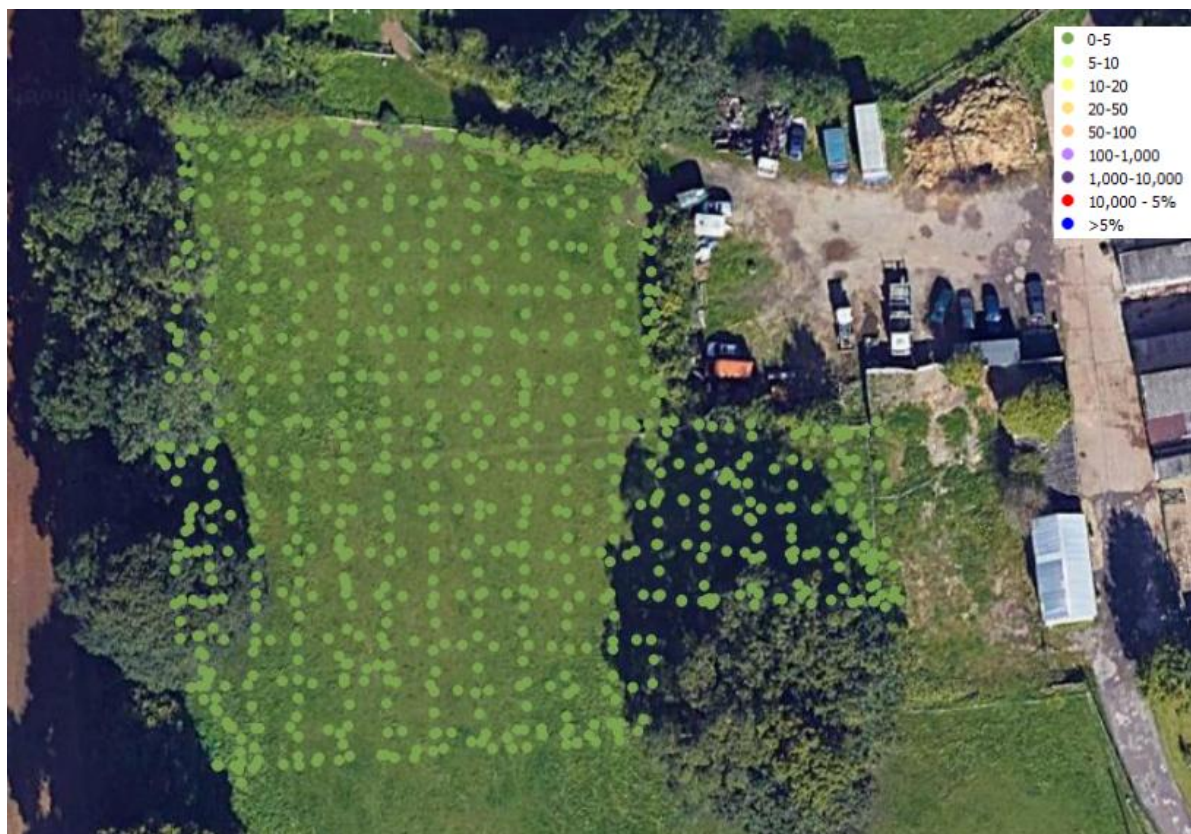
Figure 14: Surface emissions survey results
