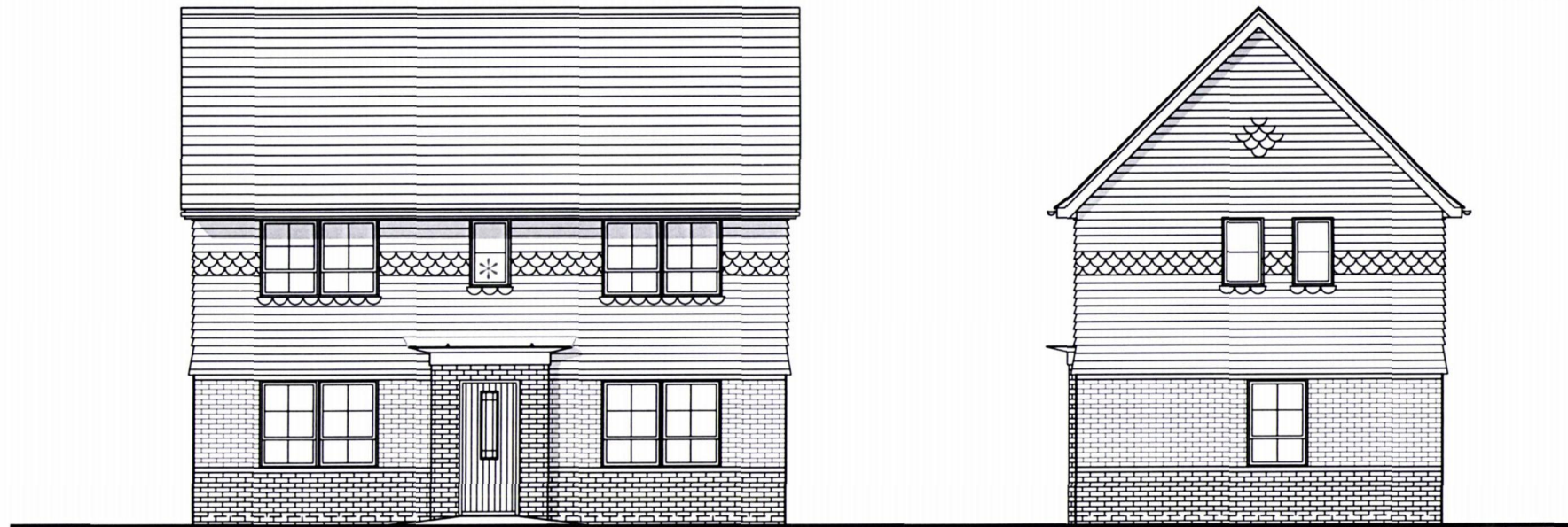
FRONT ELEVATION * Obscure Glazed Windows
