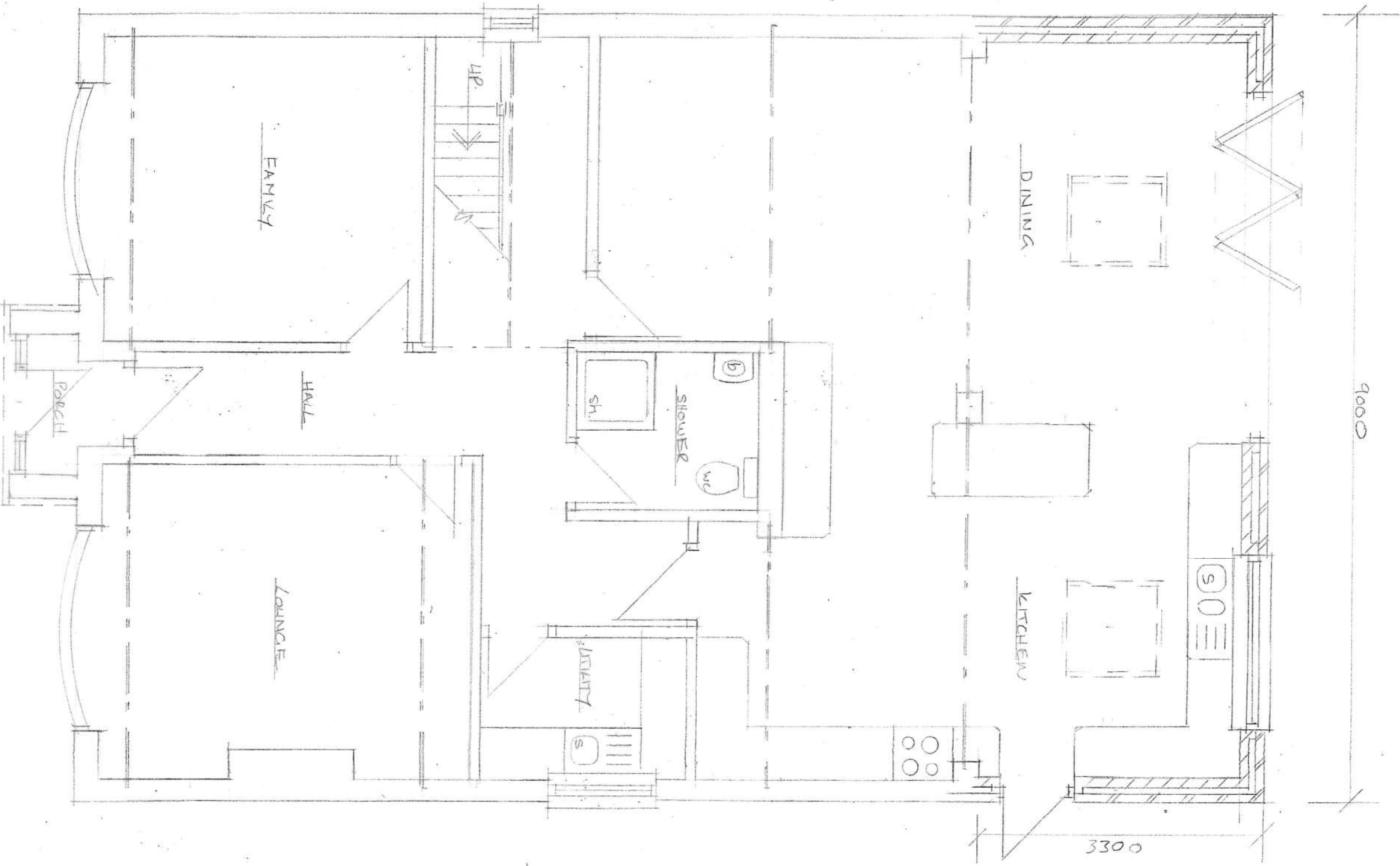
PROPOSED GROUND FLOOR PLAN. 1:50
