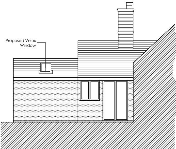
Proposed North Elevation (Within Courtyard) @ 1:100
