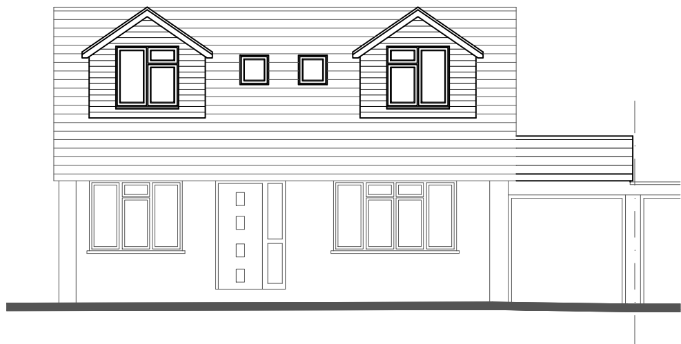
Proposed Front Elevation (scale 1:100)
