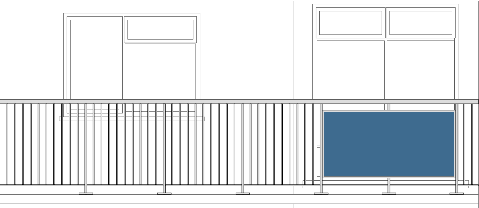
PROPOSED BALCONY RAILING TYPE 2
