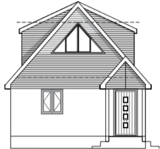
Proposed front elevation showing 'catslide' dormers either side of the ridge but above the wall plate and eaves position
