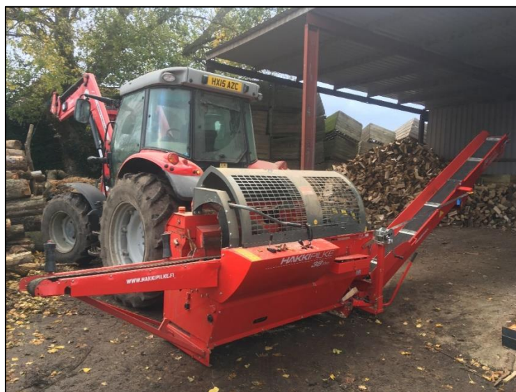
Figure 1. Firewood Processor connected to Tractor
