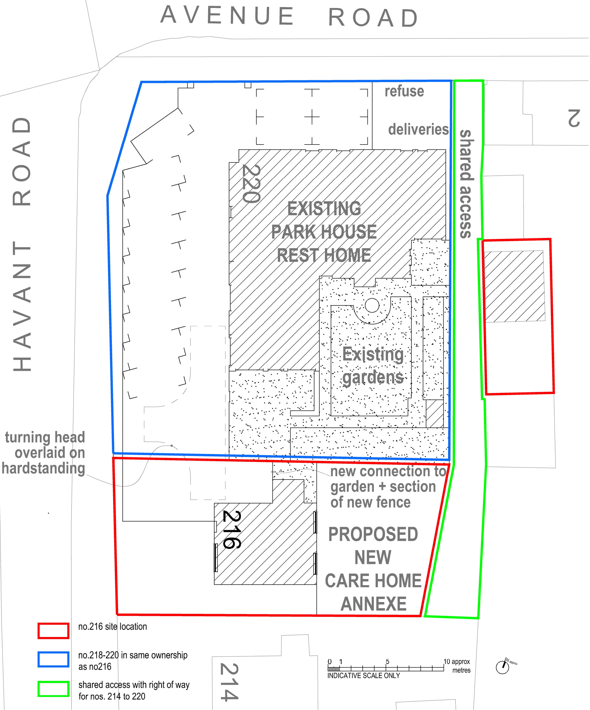
PROPOSED SITE PLAN WITH NEW PARKING LAYOUT OVERLAID ON EXISTING HARDSTANDING
