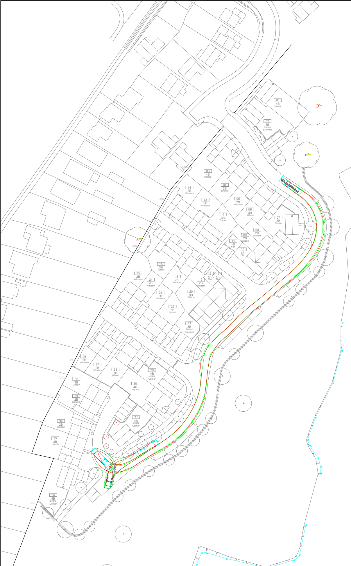
REFUSE VEHICLE TURNING ON SITE (SCALE 1:1000)
