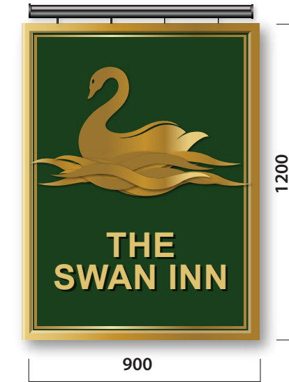
ITEM C1 ONE NEW DOUBLE SIDED PICTORIAL PANEL FITTED TO EXISTING POST ILLUMINATED BY LINOLITES Height above ground 3m
