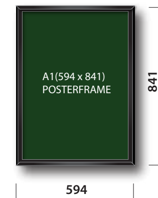
ITEM C2 TWO NON ILLUMINATED POSTER CASES FITTED TO EXISTING POST Height above ground 1.4m
