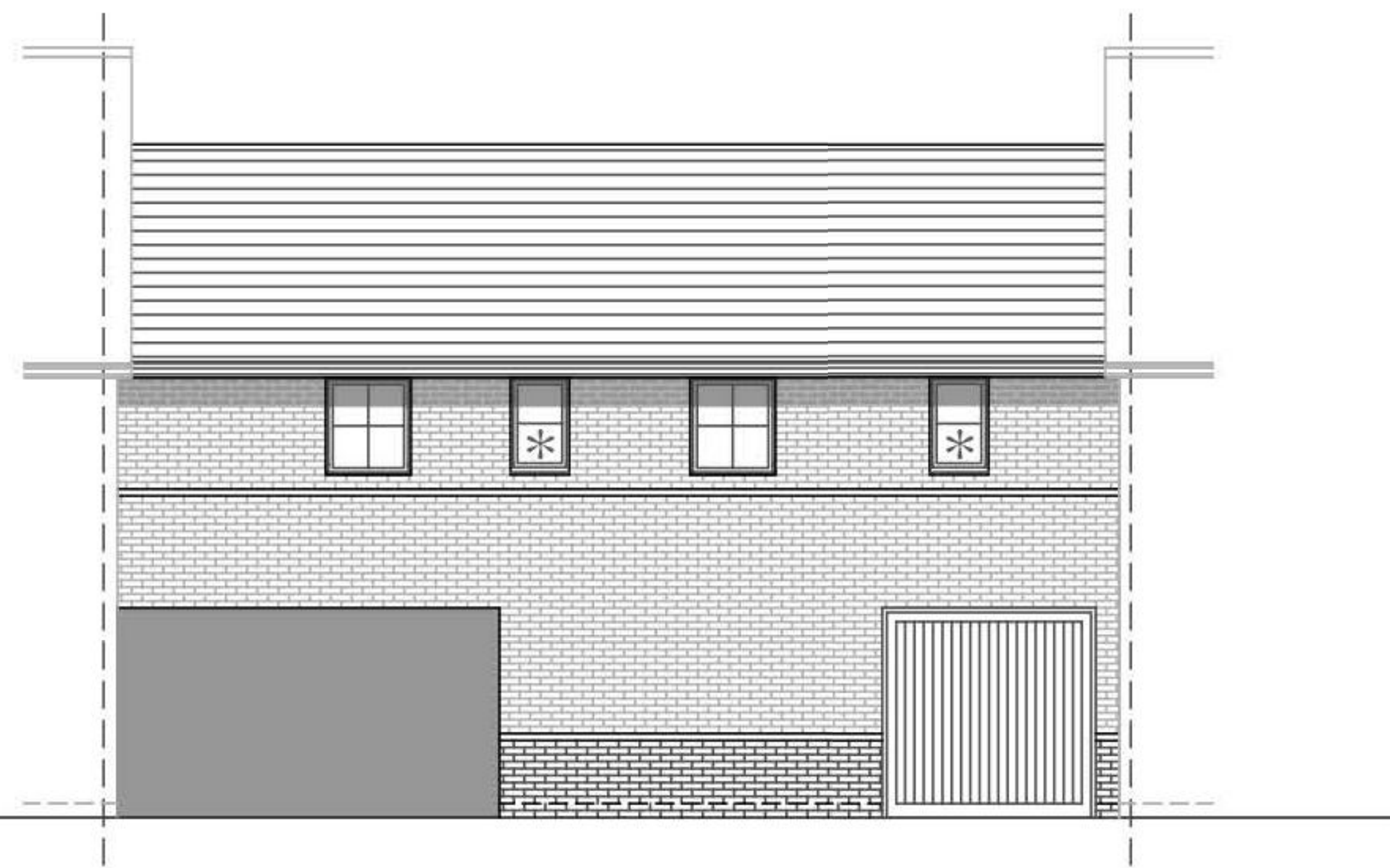
REAR ELEVATION * Obscure Glazed Windows
