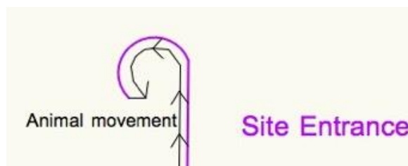
Figure 5 – ‘Cut backs’ used to guide animals away from the site entrance and where the boundary fencing meets the hard standing of the adjacent Main road.
