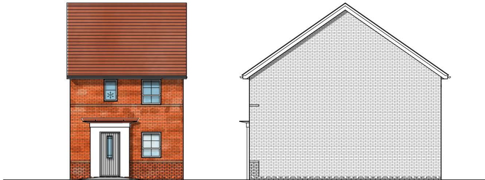
FRONT ELEVATION * Obscure Glazed Windows
