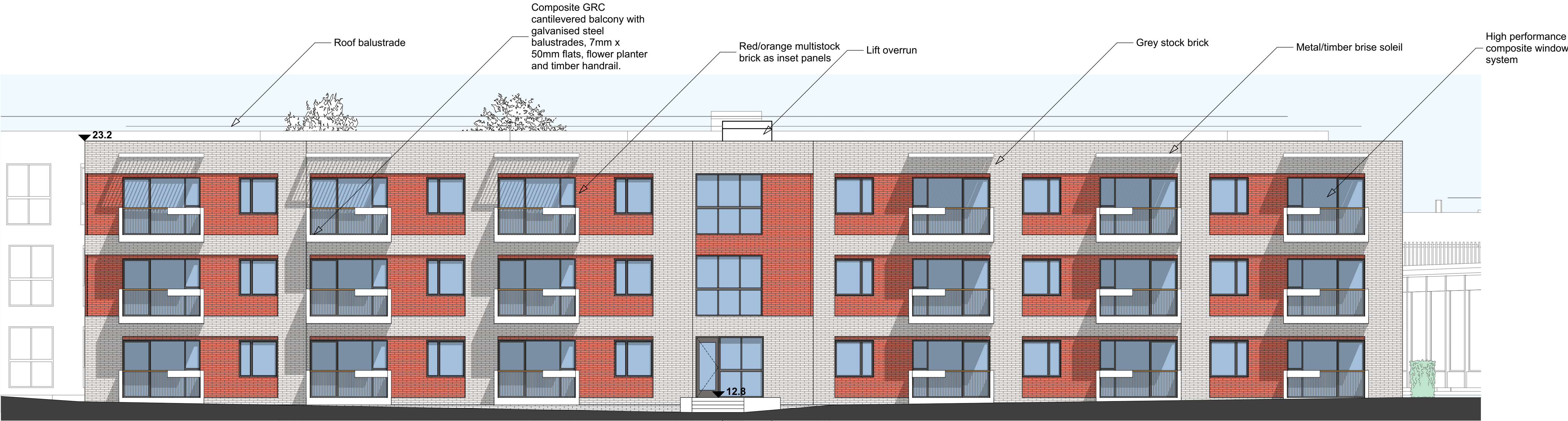
325 Supported Living East Elevation 1:100
