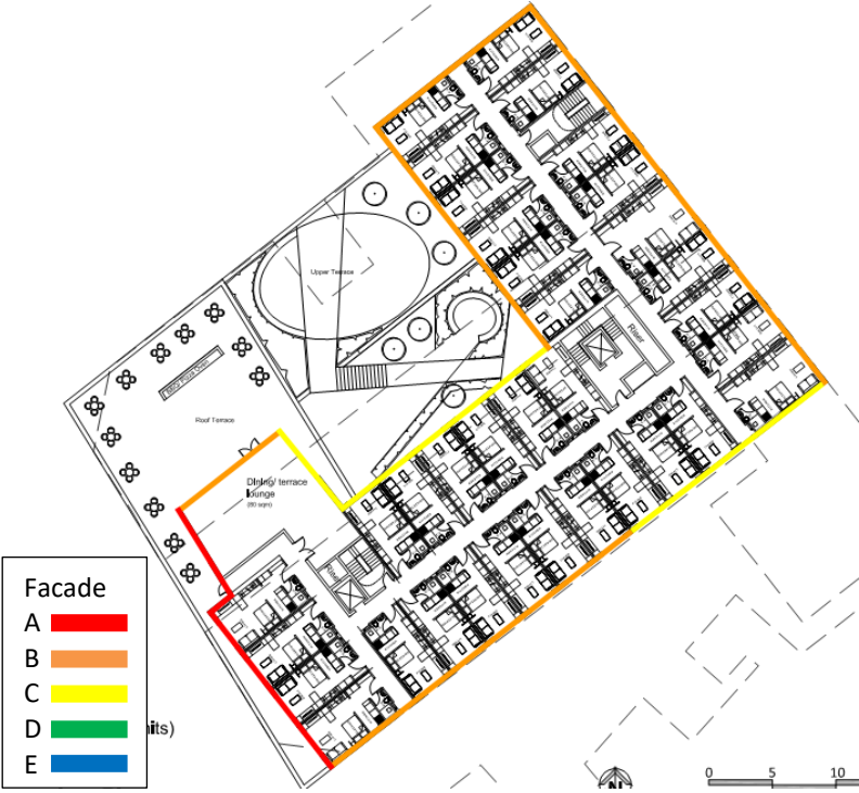
Figure 10 Mark-up of predicted facade noise levels – level 4
