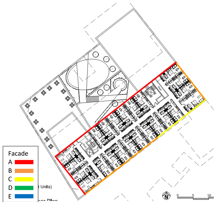
Figure 11 Mark-up of predicted facade noise levels – levels 5-8
