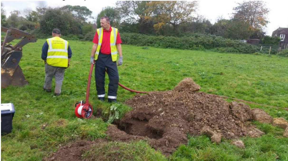
Photo 6: BRE 365 soakage tests performed
