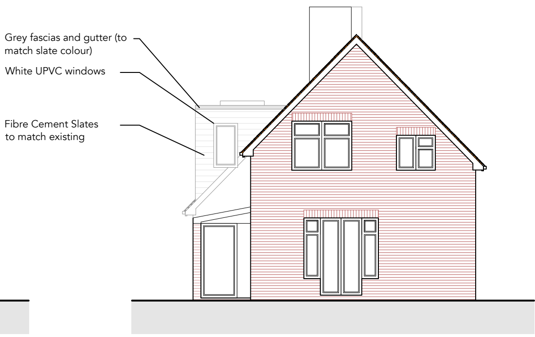
PROPOSED REAR // WEST ELEVATION 1:100
