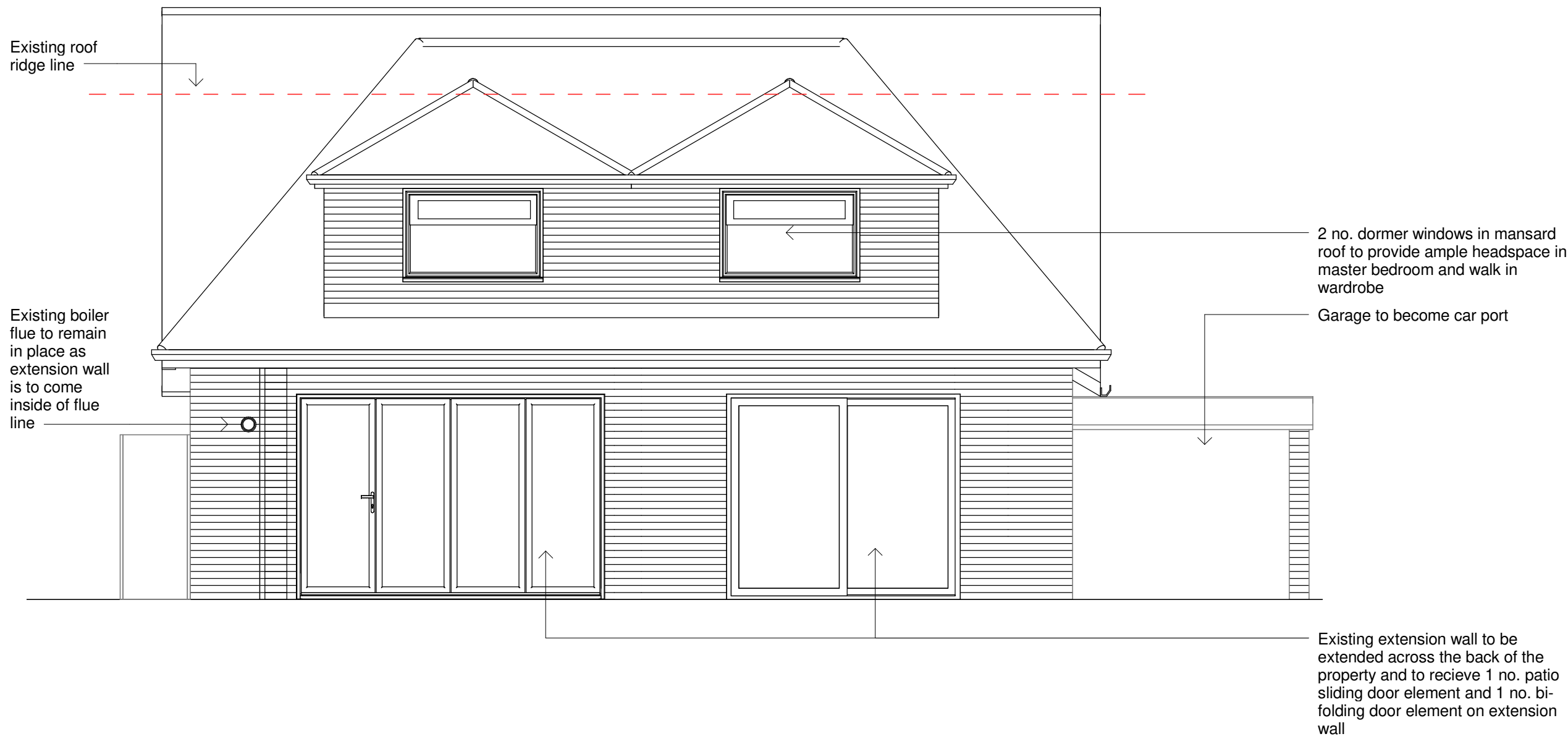
2 North West Elevation 1 : 50
