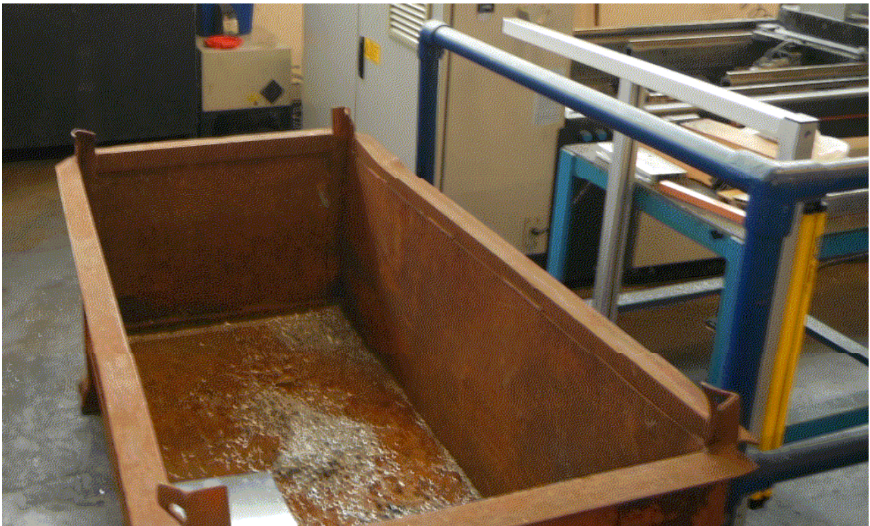
Photo 18 - Bin containing aluminium fines
