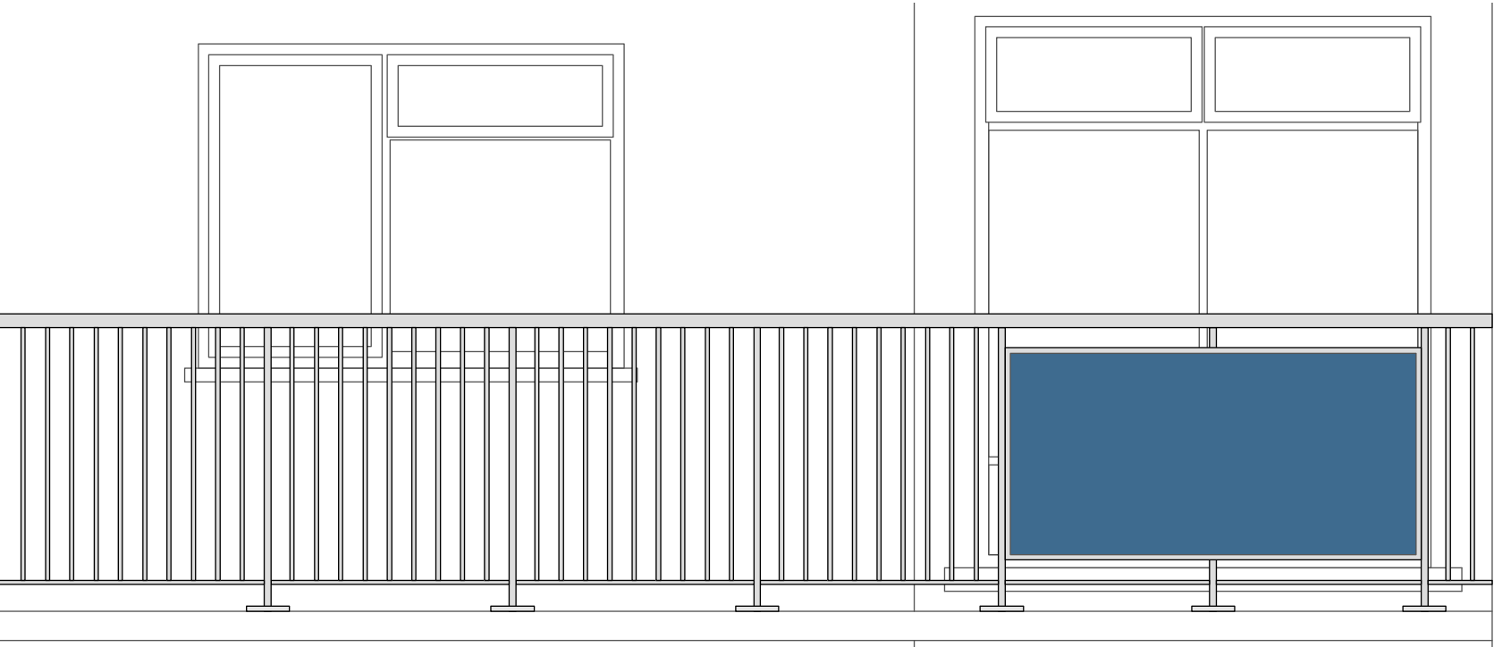
PROPOSED BALCONY RAILING TYPE 2
