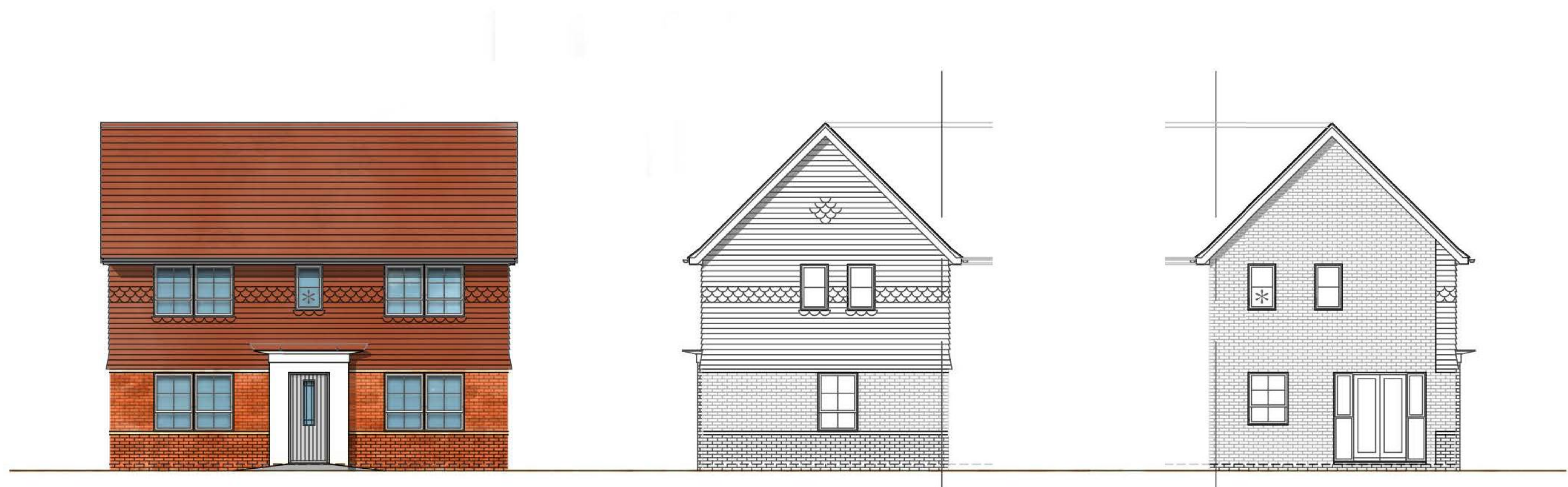
FRONT ELEVATION * Obscure Glazed Windows
