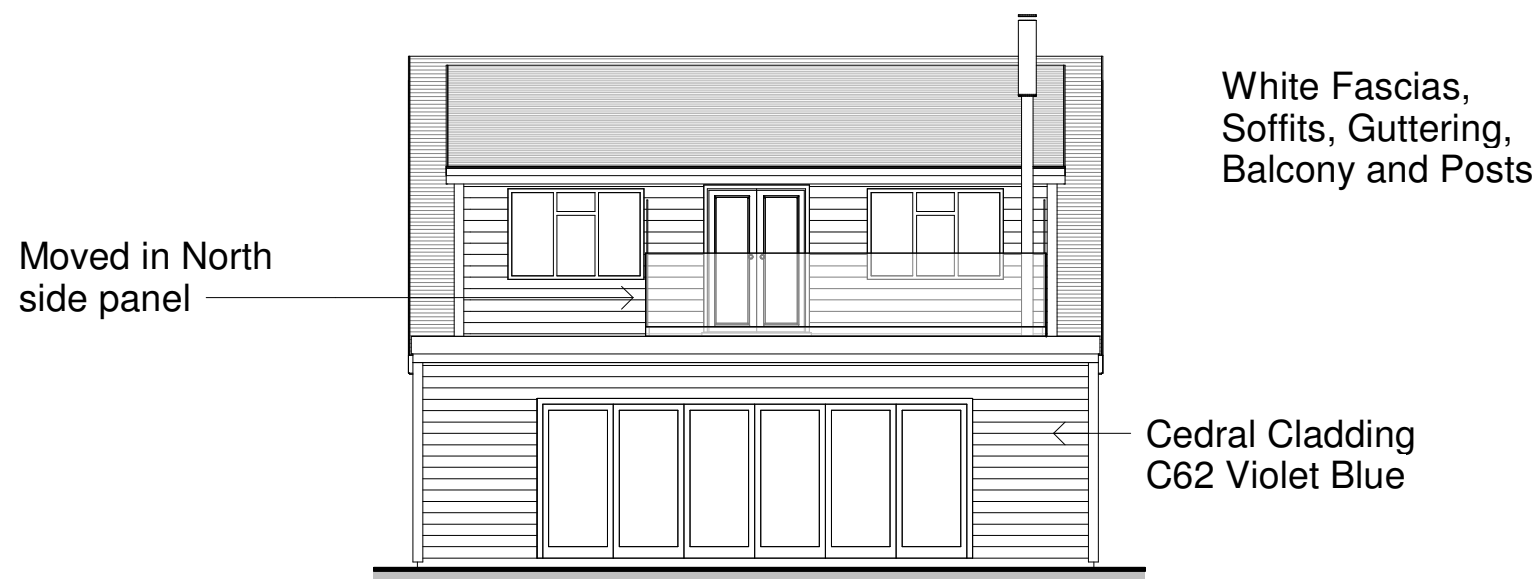
Proposed West Elevation 1 : 100
