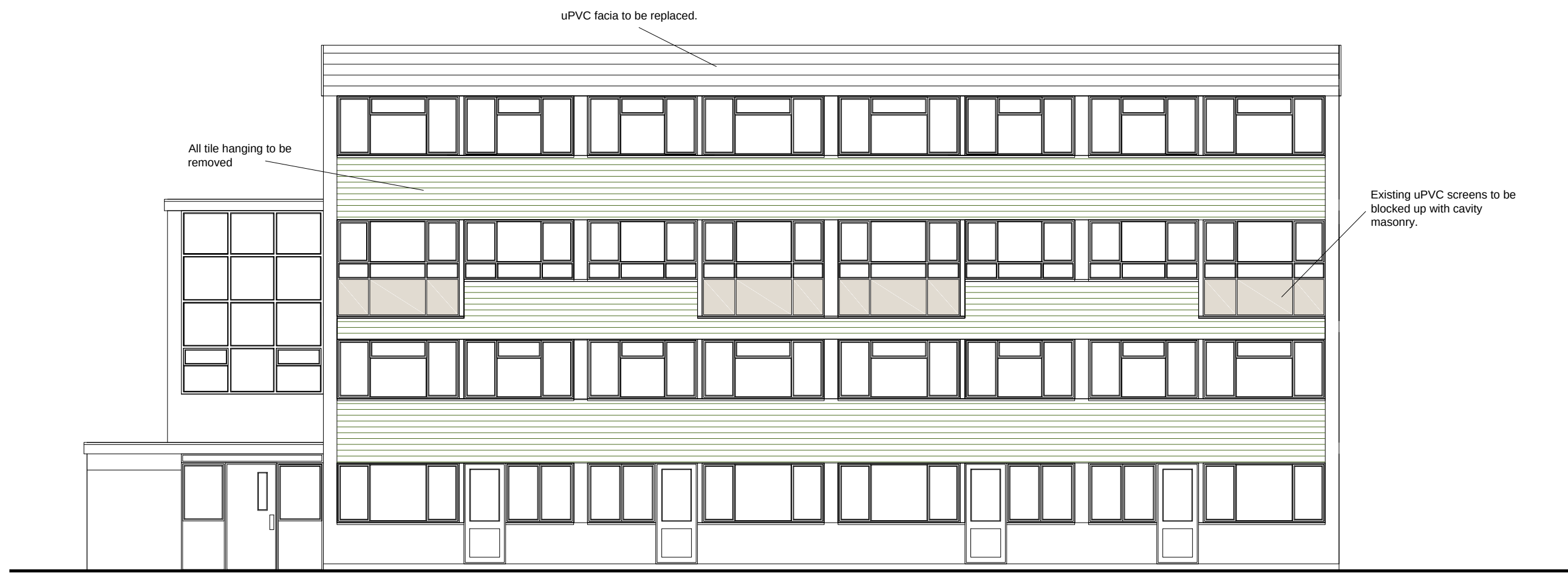
Existing Front Elevation 1:100
