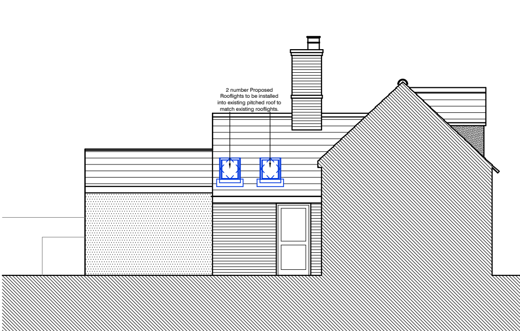
Proposed North Elevation (Inside Courtyard) @ 1:100 (A1)
