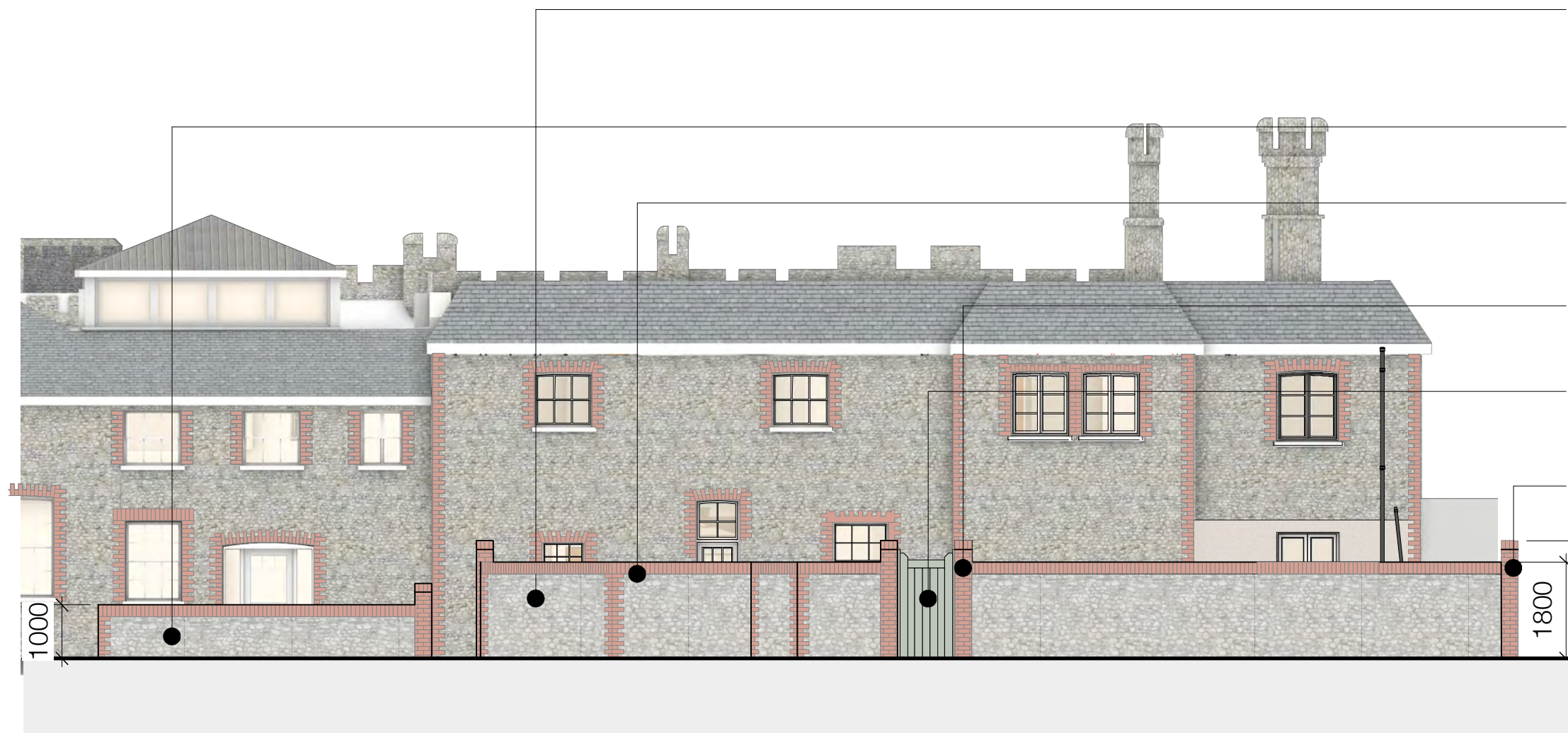
Flint wall reconstruction detail - 1:100 (north of Main House west wing)
