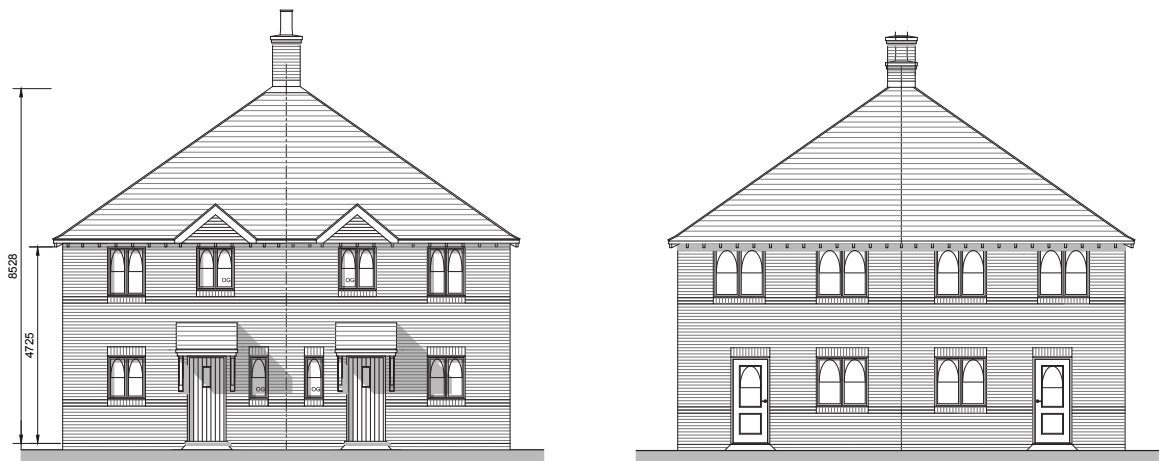
Plots 15-16 - Affordable dwellings designed as a lodge building adjacent to East Leigh house
