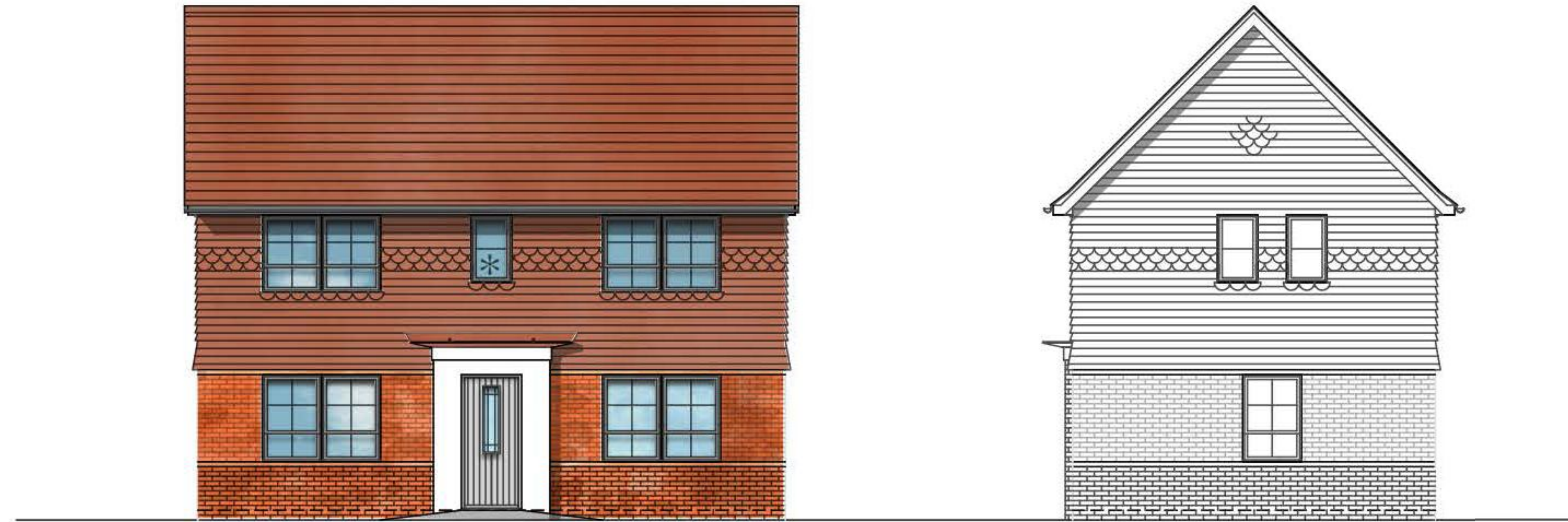
FRONT ELEVATION * Obscure Glazed Windows
