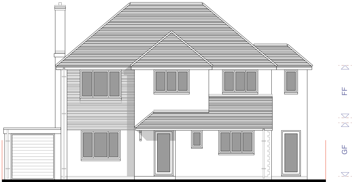
Proposed East (Front) Elevation at 1:100 scale
