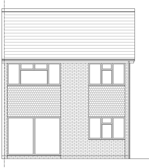
EXISTING REAR ELEVATION
