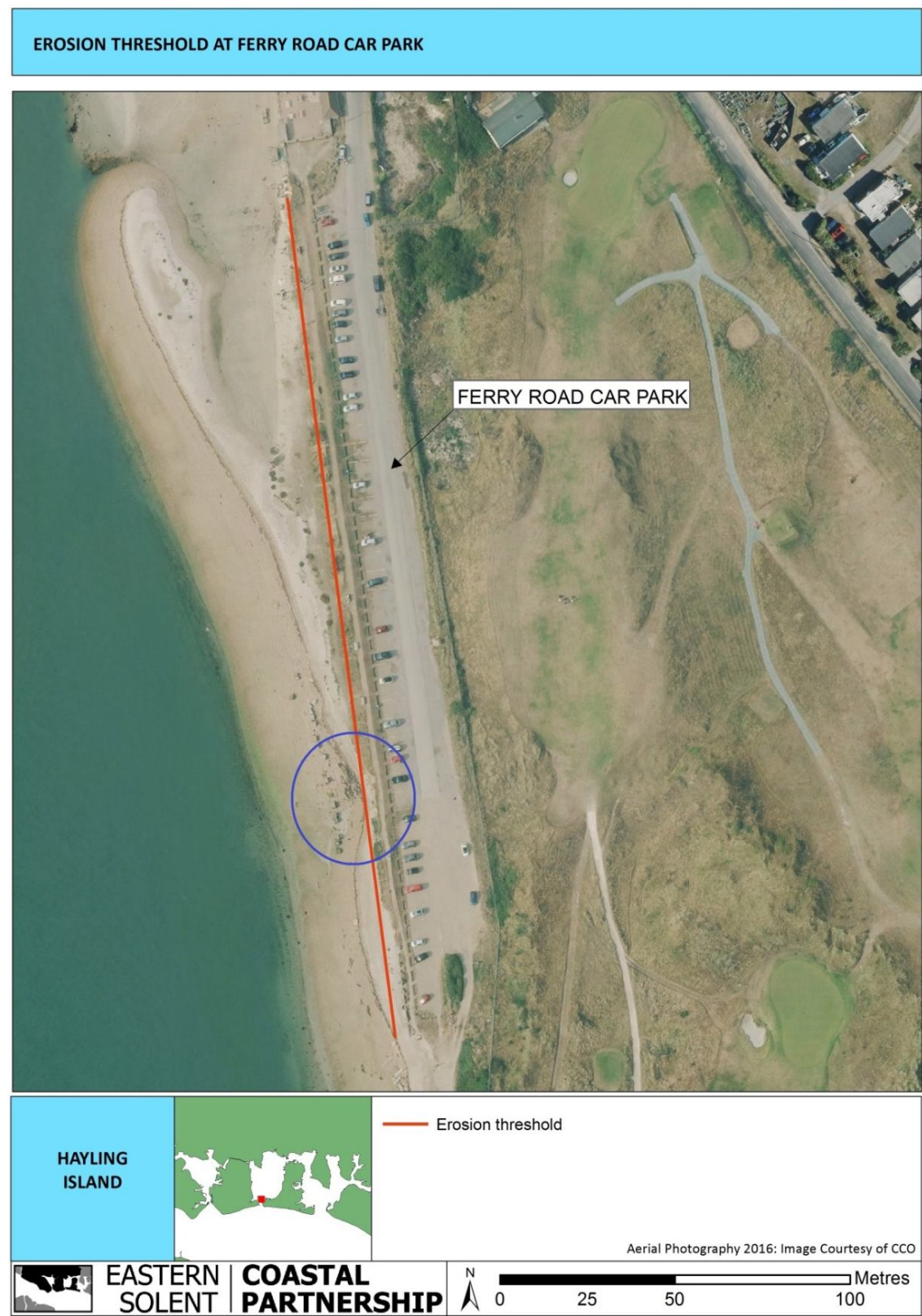
Figure 3.5 Erosion threshold at Ferry Road car park, Hayling Island. The hotspot of erosion currently present is circled in blue
