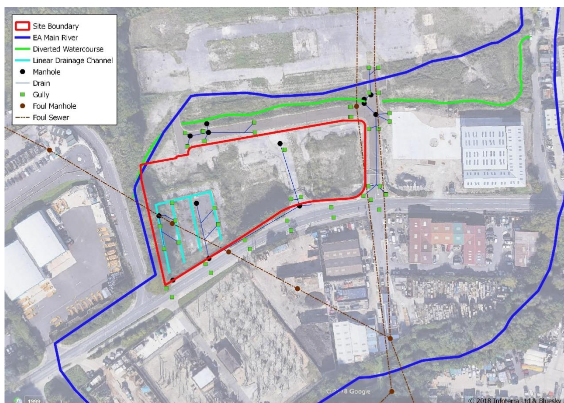
Figure 7 Existing Drainage Features
