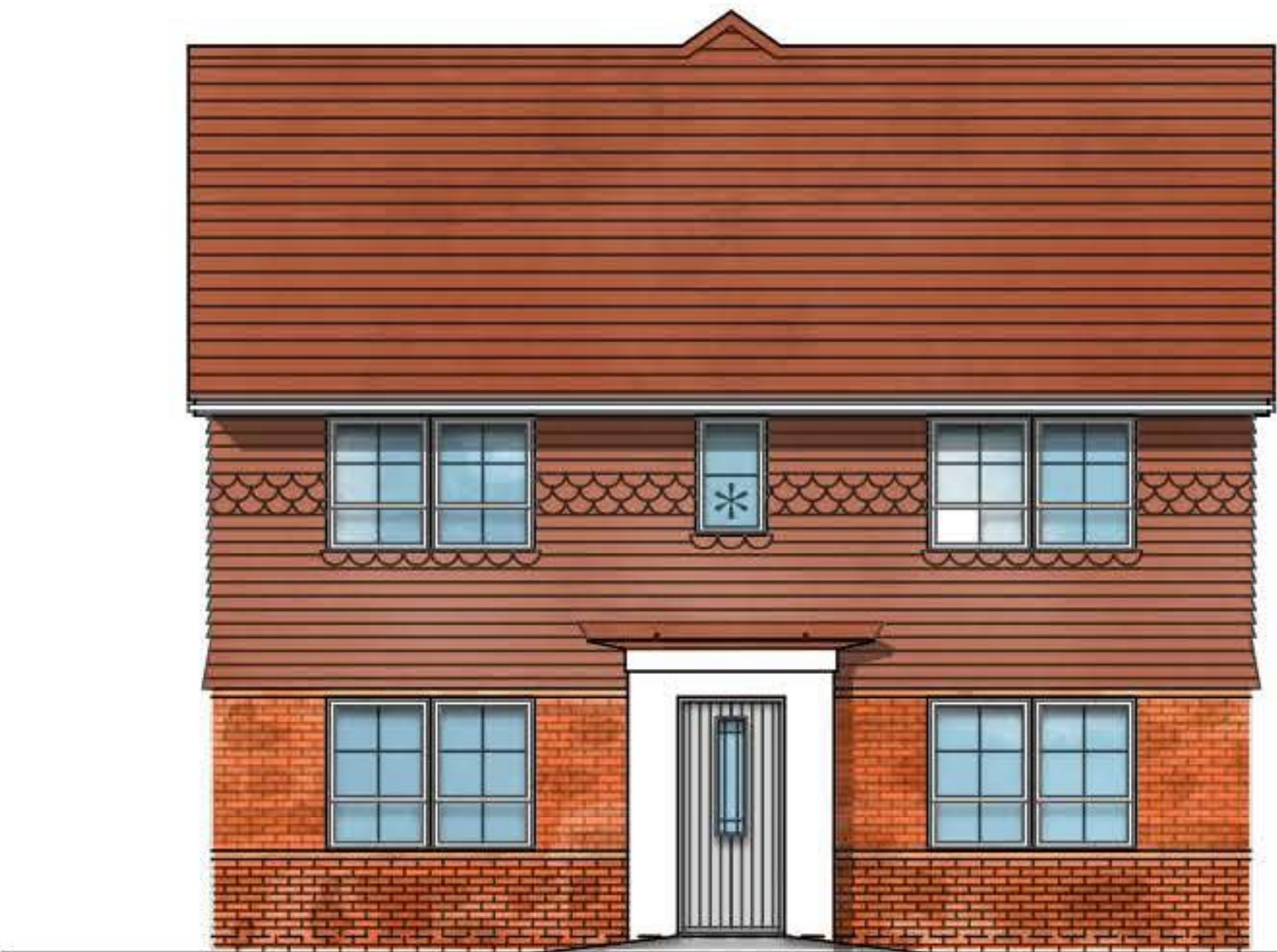
FRONT ELEVATION * Obscure Glazed Windows
