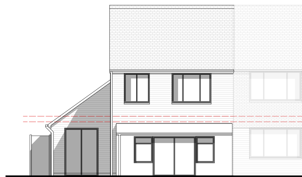
East Elevation (Existing) 1:100
