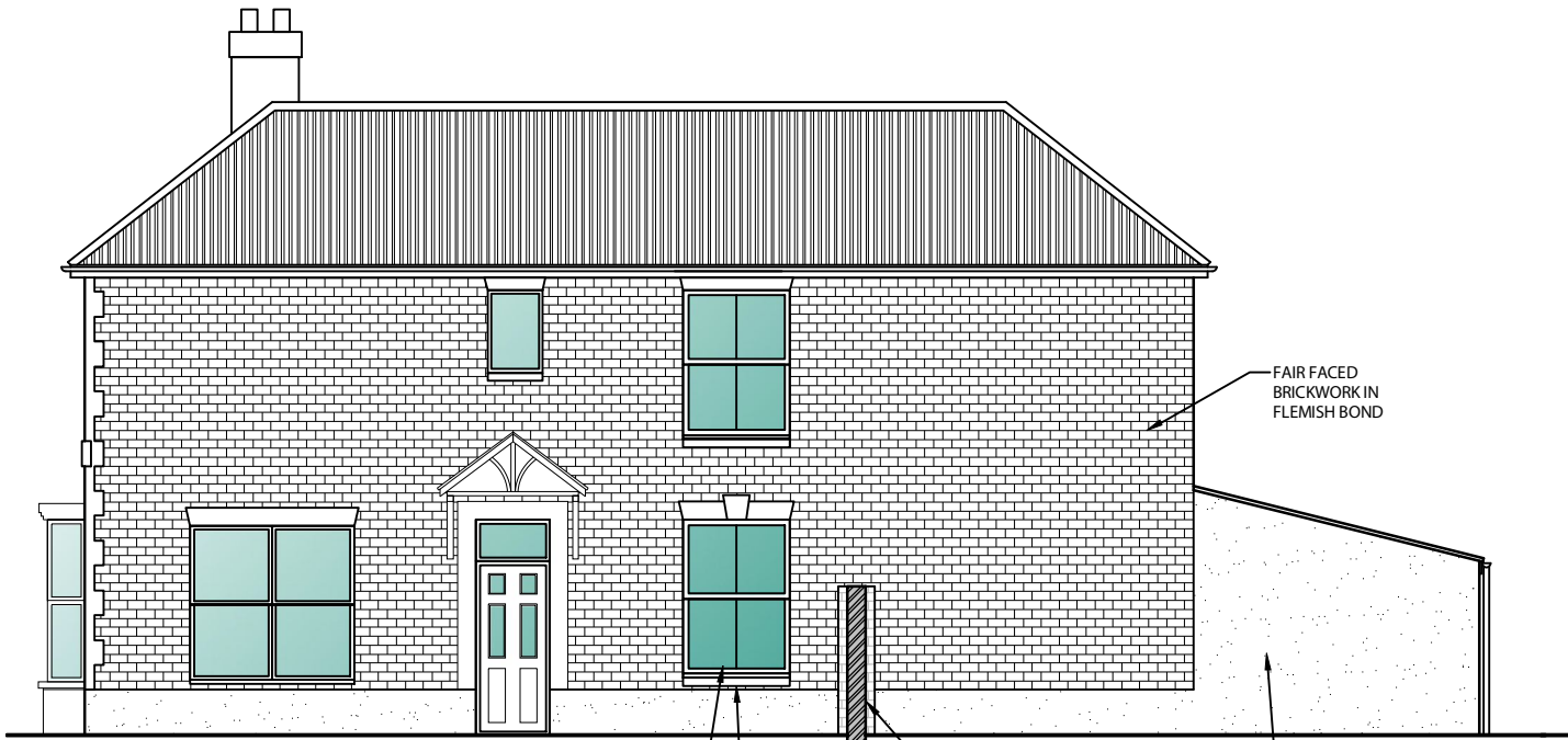
EXISTING SIDE ELEVATION
