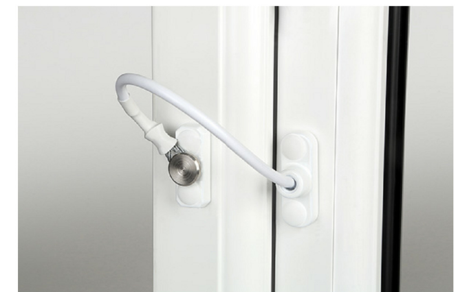
Proposed restrictor "Jackloc Swivel/Stud" permanent window restrictor, installed to restrict opening to 50mm
