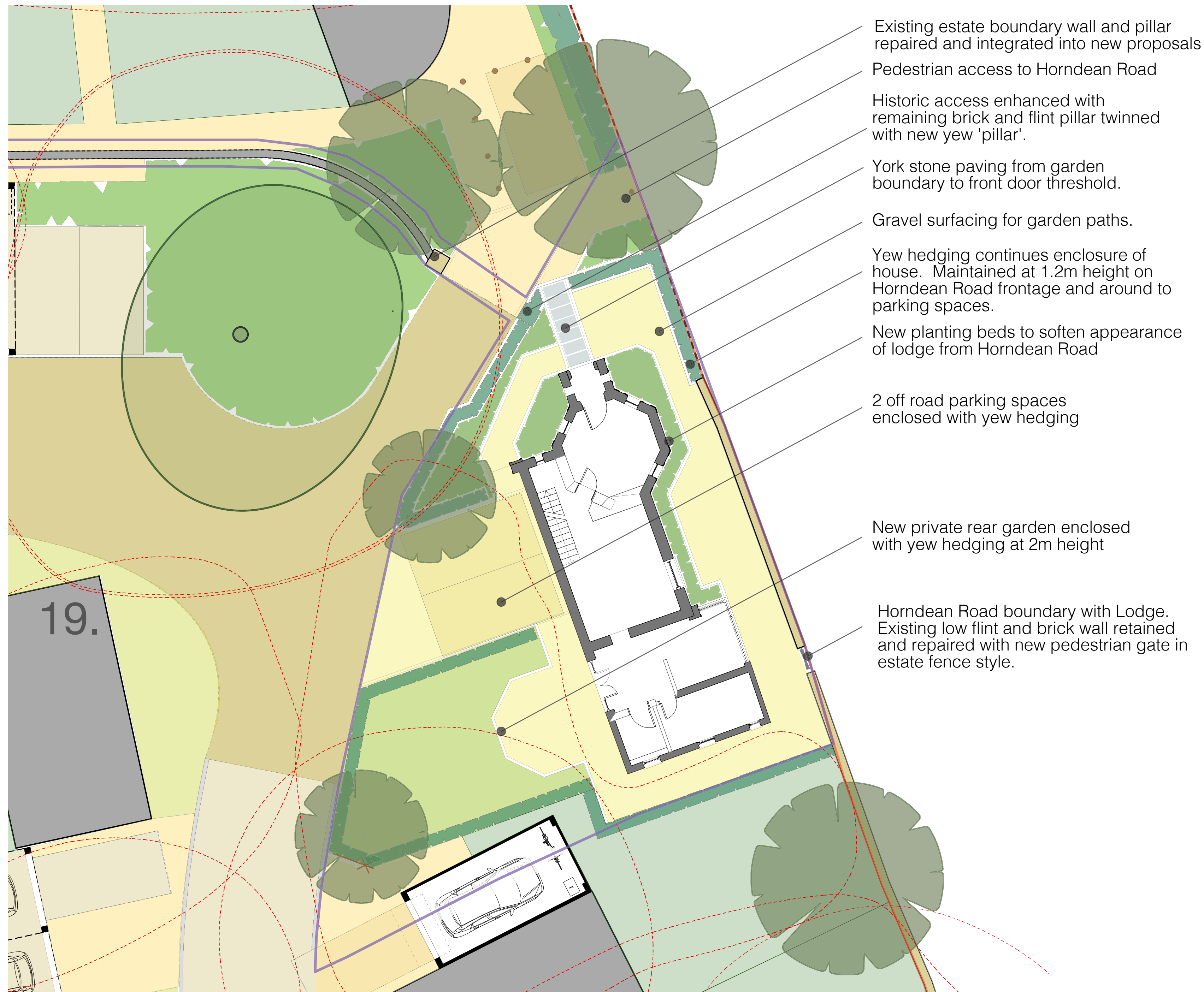
Lodge boundary wall with Horndean Road. Security fencing will be removed, the wall repaired and a new estate style gate installed
