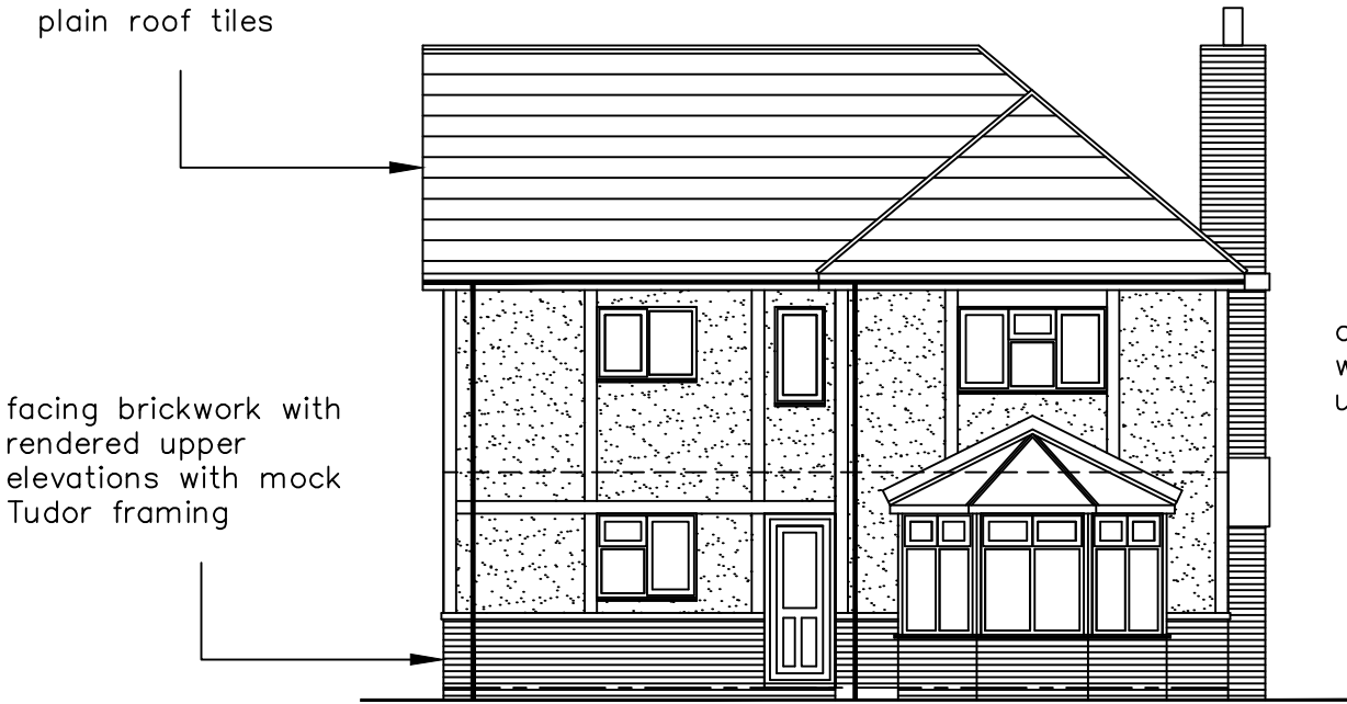
EXISTING EAST ELEVATION
