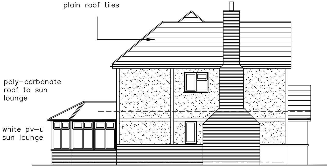
EXISTING NORTH ELEVATION
