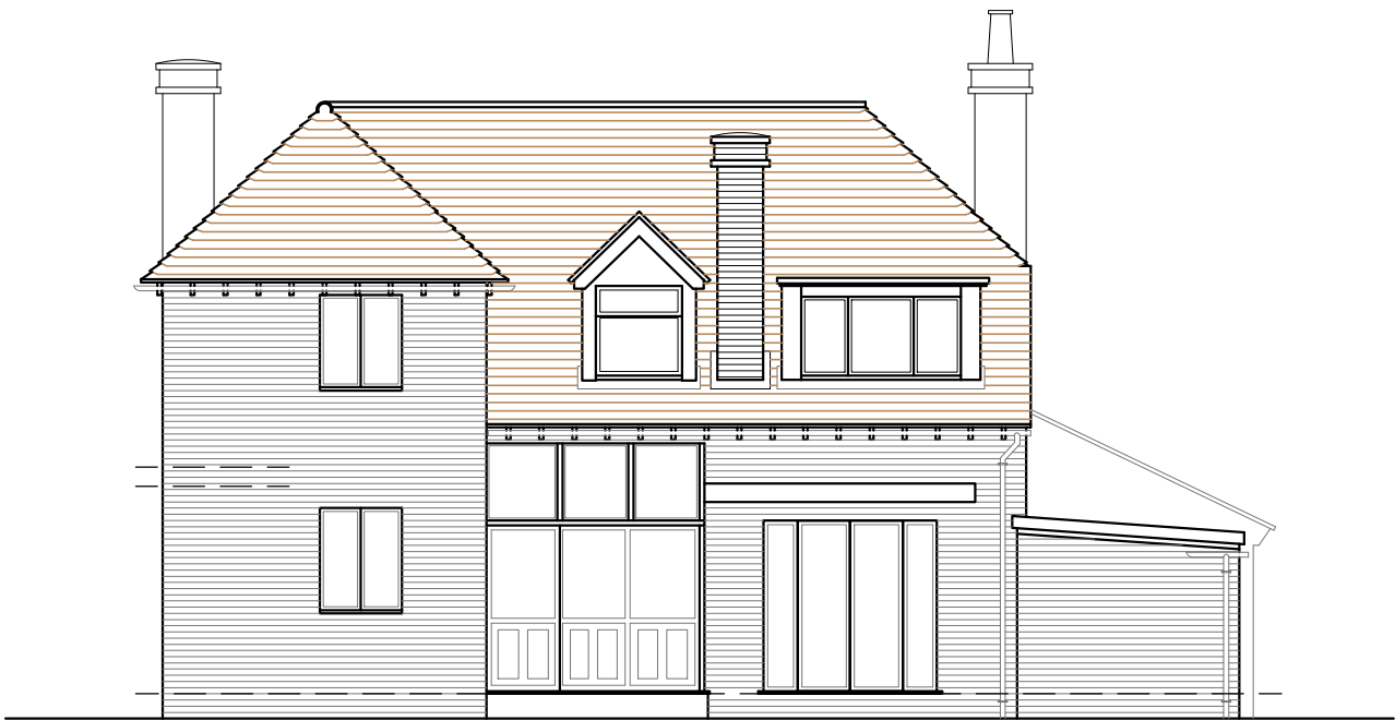
Existing East Elevation @ 1:100
