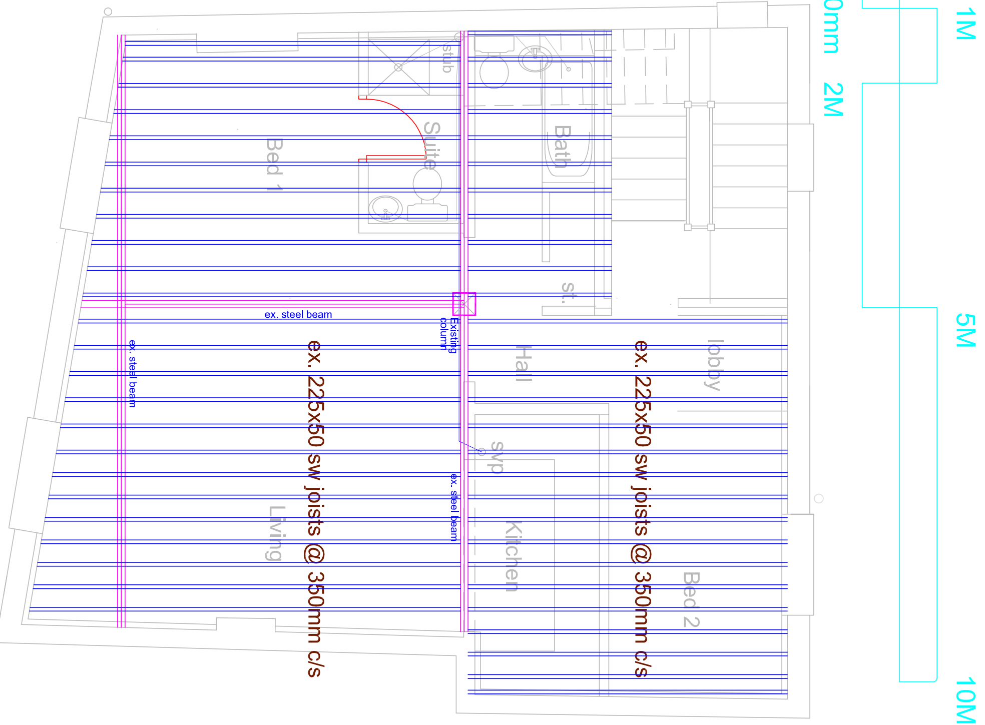
UPPER FLOOR JOISTS
