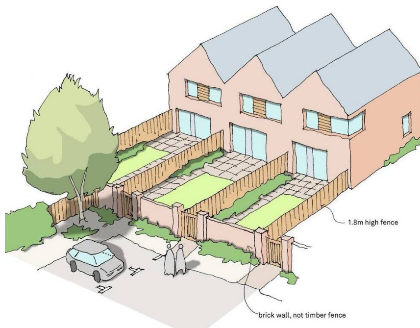
Figure 4.12: Appropriate boundary structures for rear private gardens
